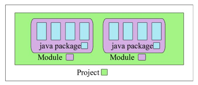
With the introduction of the module system, the JDK was reorganized into 94 modules. Java applications can use the newly added **jlink tool** (Jlink is a new command-line tool released with Java 9. It allows developers to create their own lightweight, customized JRE for module-based Java applications) to create custom runtime images that only contain the required JDK modules. This significantly reduces the size of the Java runtime environment.
