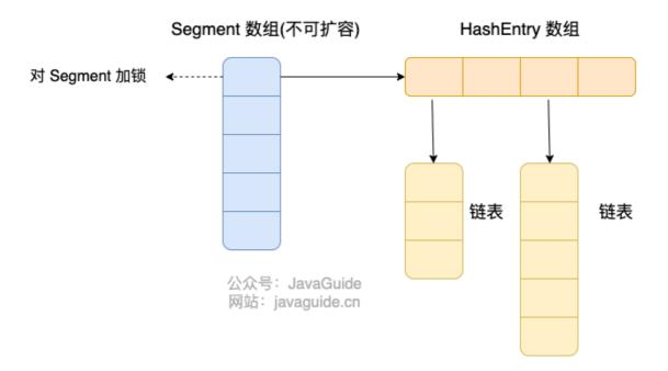
In JDK 1.8, segmented locking ConcurrentHashMap was removed and concurrency safety was ensured. The data structure is similar to that of 1.8: array + linked list/red-black binary tree. Java 8 converts the linked list (with an addressing time complexity of O(N)) to a red-black tree (with an addressing time complexity of O(log(N)))) when the linked list length exceeds a certain threshold (8). Segment Node + CAS + synchronized HashMap
