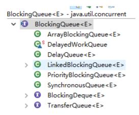
The following mainly introduces three common BlockingQueue implementation classes: ArrayBlockingQueue, LinkedBlockingQueue, and PriorityBlockingQueue.
