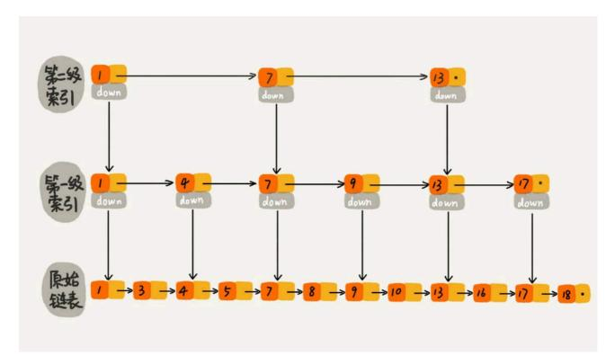
The lowest level linked list maintains all the elements in the skip list, and each upper level linked list is a subset of the lower level.
