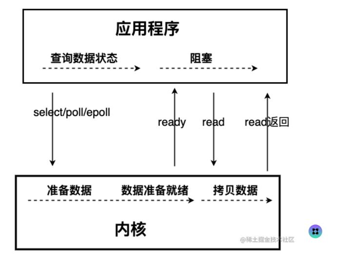
In the I/O multiplexing model, a thread first initiates a select call to query the kernel whether the data is ready. Once the kernel has the data ready, the user thread initiates a read call. The read call process (data transfer from kernel space to user space) is still blocking.
