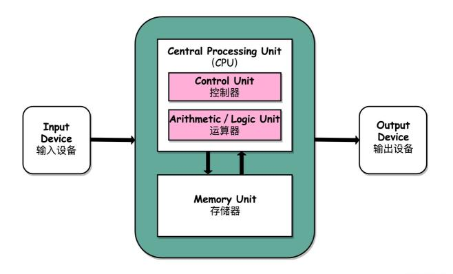
Input devices (such as keyboards) and output devices (such as monitors) are both external devices. Network cards and hard drives can be considered both input and output devices.
