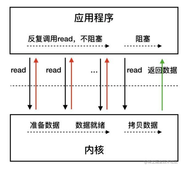
In the synchronous non-blocking IO model, the application will continue to initiate read calls, waiting for the data to be copied from the kernel space to the user space. During this time, the thread is still blocked until the kernel copies the data to the user space.
